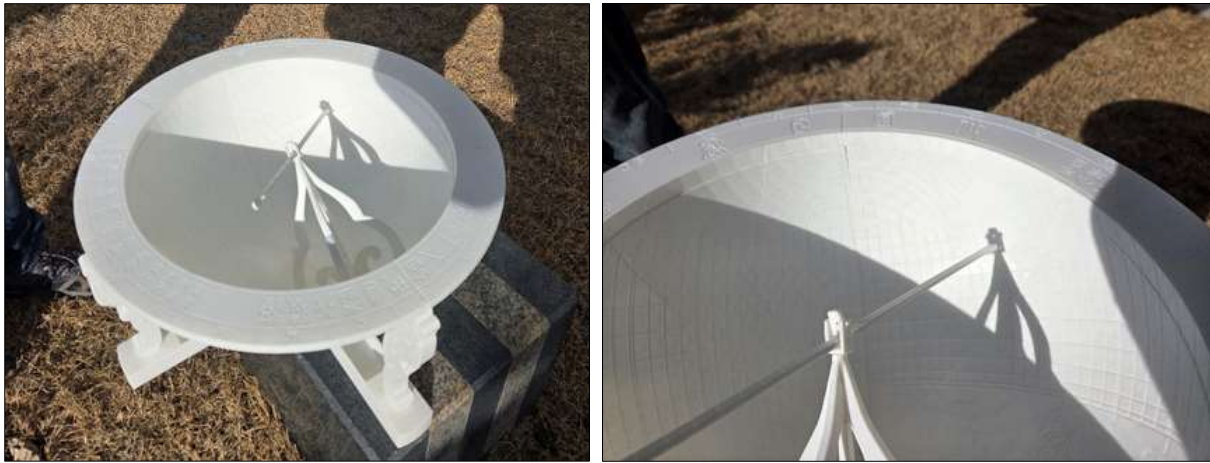
Figure 4: 3D-printed model of the Sejong Angbu-ilgu in this research; (left): scene estimating time; (right): sunlight passing through the pinhole projected on the hemisphere (photographs: the authors).
