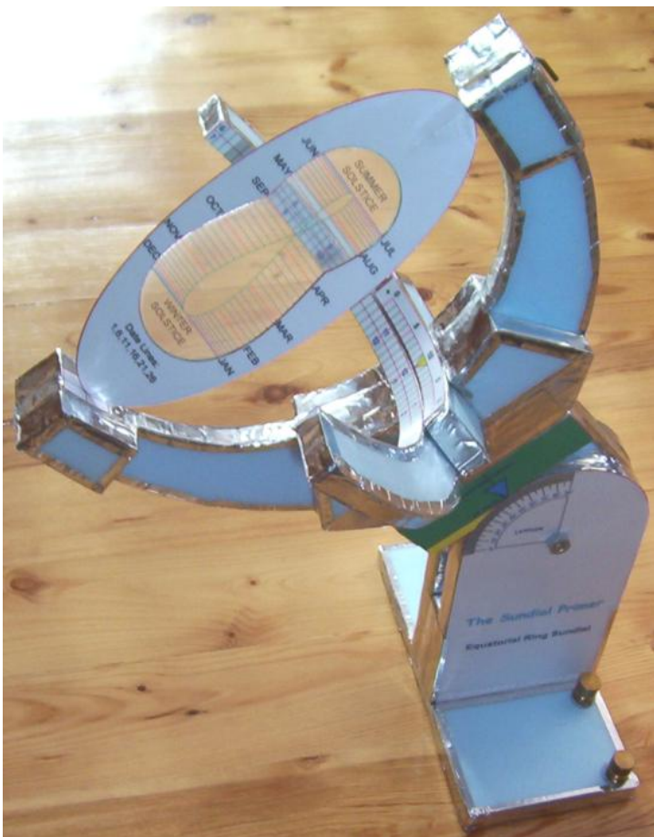
Standard Time Equatorial Ring Sundial - Transparent Analemmic Gnomon
