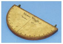
6-1/2" (17 cm) diameter mahogany semicircle is mounted with the manuscript angular scale running 90-0-90 by degrees, pierced brass sight vanes, and brass mounting hole for plumb bob line. It is a rare form, like the sighting quadrant but doubled for measuring both elevation angle and depression angle, and is in very fine condition throughout. The maker is not recorded in the standard references, but apparently worked in Stockton near Stratford-on-Avon. \$850.
