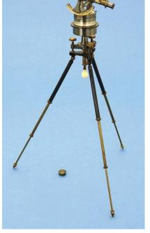
compass has needle arrester and circumferential degree scale on silver divided 0(4)360. The little telescope has racked focus and optics within. There are crossed adjustable spirit levels, and sight vanes below. The instrument is mounted to a three-screw leveling
