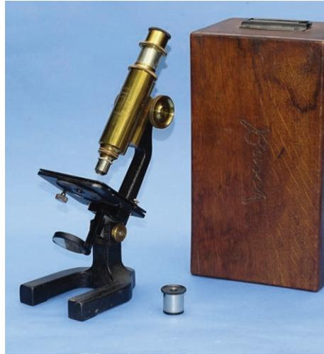
7. **STUDENT MICROSCOPE FROM EASTERN GERMANY**, c. 1930, signed "Busch, Rathenow, Germany, Nr. 16003" on the main tube, and "Busch" on the two oculars, the objective, and the case. Extending from 10-1/2" to 15" (27 - 38 cm) by drawtube and racked coarse focus, the microscope has horseshoe base, hinged limb, unusual tilting-stage fine focus, substage wheel of stops and double mirror. A good example in very fine condition, constructed of black enameled iron and bright lacquered brass. \$380.
