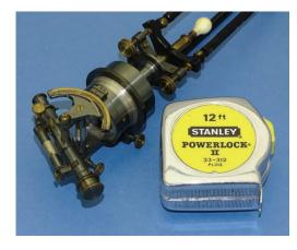
26. EXQUISITE SUB-MINIATURE FULLY-FUNCTIONING THEODOLITE, French, c. late 19th century, the theodolite itself standing 2-1/2" (6 cm) tall, of chemically blackened and bright lacquered brass. The 31 mm diameter azimuthal scale is divided on conical canted silver, every degree 0-360, and with twin one-arcminute verniers. The vertical altitude scale is divided every degree 0+/-60, with four-arcminute vernier. The motions have clamps and spring-loaded fine motion tangent screws. A central glazed
