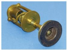
8. UNUSUAL VERTICAL PILLAR-SCREW-FOCUS MICROSCOPE, c. late 18th century. Made of brass with turned hardwood base, its height extends from 5" to 6" (13-15 cm, this the range of focus) by unusual threaded pillar supporting the microscope's twin columns to its twin-lens optical tube. Atop the threaded pillar is the stage plate, which carries an extending support for an (absent) stage accessory. Condition is fine. A thread around the base suggests it once had a domed cover.
