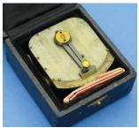
20. "L'EQUERRE-GRAPHOMETRE AMAGAT" – A POCKET SEXTANT-FORM SURVEYING INSTRUMENT, French, c. late 19th century, signed "H. Morin, 11 rue Dulong, Paris." The 3" (8 cm) square darkened brass instrument has sighting port, adjustable "horizon" mirror, and swinging "index" mirror on an arm whose position is read against 0(1)120 scale, with two arc-minute vernier. It is in excellent condition, complete with original lined case and printed description and
