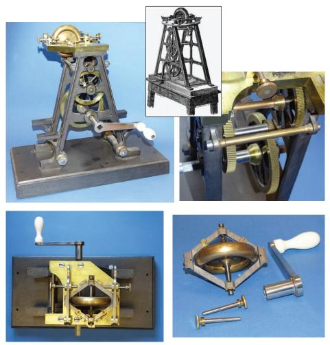
**44.** FOUCAULT GYROSCOPE AND ITS LAUNCHING TOWER, French, late 19th c., signed "E. Ducretet et L. Lejeune à Paris", constructed of brass and iron. The tower of gears stands 17" (43 cm) tall overall complete with the gyroscope assembly. The iron base measures 9" x 17-3/4" (23 x 45 cm). Condition is fine.
