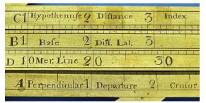
Distance Run along the hypothenuse (scale C), and the Course being the bearing angle on the quadrant scale. The Merdian Line (scale D) may be useful in Parallel sailing calculations. (see, e.g., Norie, *A New and Complete Epitome of Practical Navigation*, 1825, 8th edition).
