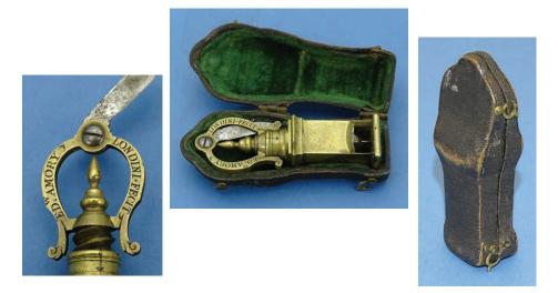
**33. EARLY VERTICAL QUILL CUTTER**, English, c. early 18th century, the fine brass and steel instrument signed "Ed'w. Amory Londini Fecit", numbered 90 on the base. Standing 2-1/2" (6 cm) tall, it features a hinged blade on top, a curved slot and shaped cutter in the body, being driven by a handle to the coarse thread. The finely shaped fitted case is bound in dark fish skin, and the whole is in very fine condition.
