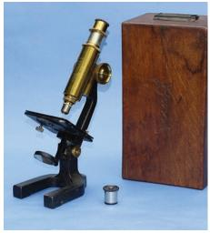
signed "Busch, Rathenow, Germany, Nr. 16003" on the main tube, and "Busch" on the two oculars, the objective, and the case. Extending from 10-1/2" to 15" (27 - 38 cm) by drawtube and racked coarse focus, the microscope has horseshoe base, hinged limb, unusual tilting-stage fine focus, substage wheel of stops and double mirror. A good example in very fine condition, constructed of black enameled iron and bright lacquered brass. \$380.
