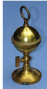
When the interior is evacuated, the hemispheres are forced together by the surrounding air, resisting efforts to separate them. Invented c. 1650 in Magdeburg by Otto von Guericke, the hemispheres are a fundamental demonstration of atmospheric air pressure. \$350.
