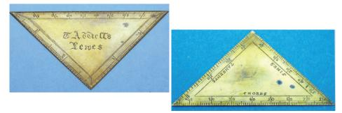
36. UNUSUAL MATHEMATICAL TRIANGLE, English, c. 19th century, signed "T.A. Wells(?), Lewes." With a 4-1/4" (11 cm) long edge, this right triangle has, on the front, a 90° protractor on the hypotenuse, and inch scales on the short sides by tenths and by twelfths. The reverse is divided with edge scales of Sines, Tangents, and Chords. In fine condition, it is a most unusual mathematical tool by this unrecorded craftsman from the south of England.
