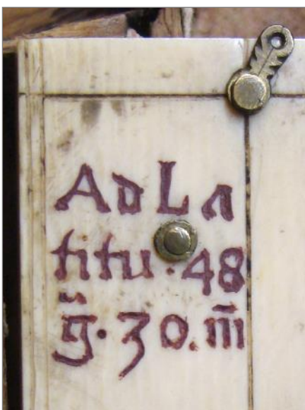
Fig. 2. One of numerous explanatory labels on the quadrant, this one specifying that it has been designed for use at latitude 48° 30'.
