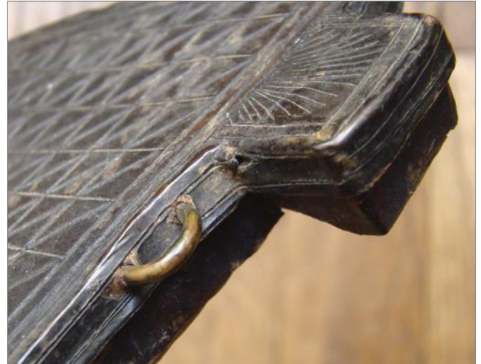
Fig. 7. Details showing the case-work extension for a sight vane, plus one of the original brass eyes for cord to bind and carry the instrument.
