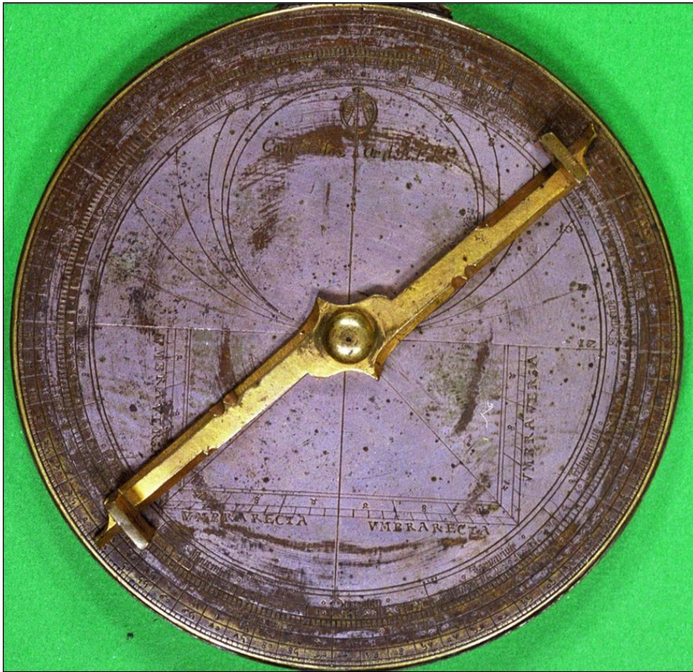
Figure 2: The alidade mounted on the back of the mater (photograph: Jacques Cadaugade).
